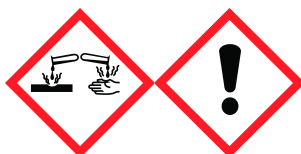
Corrosion Exclamation mark
