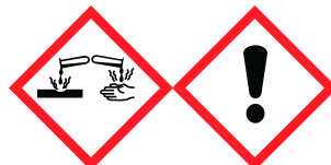
Corrosion Exclamation mark
