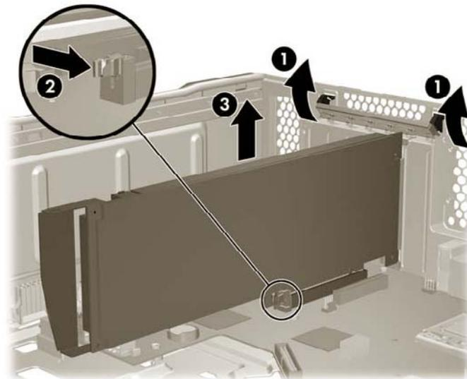
Release the card slot latch (❷), and then carefully lift the card from the chassis (❸).
