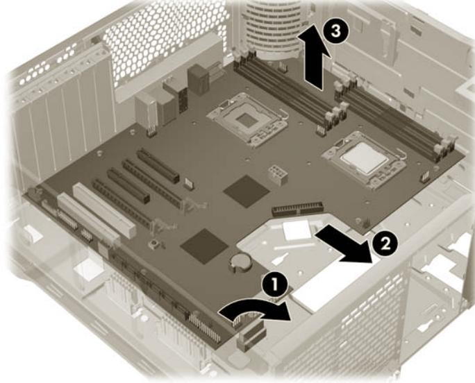
Slide the system board forward ❷, and lift it from the chassis ❸.
