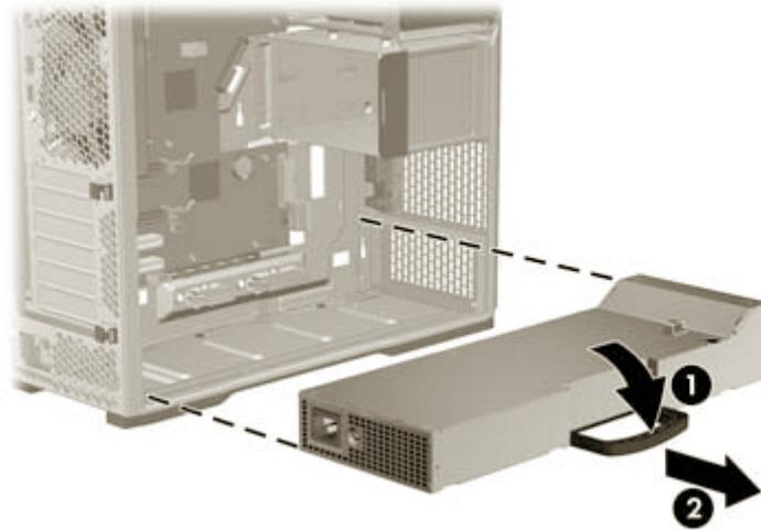
Use the handle to pull the power supply out of the chassis ❷.
