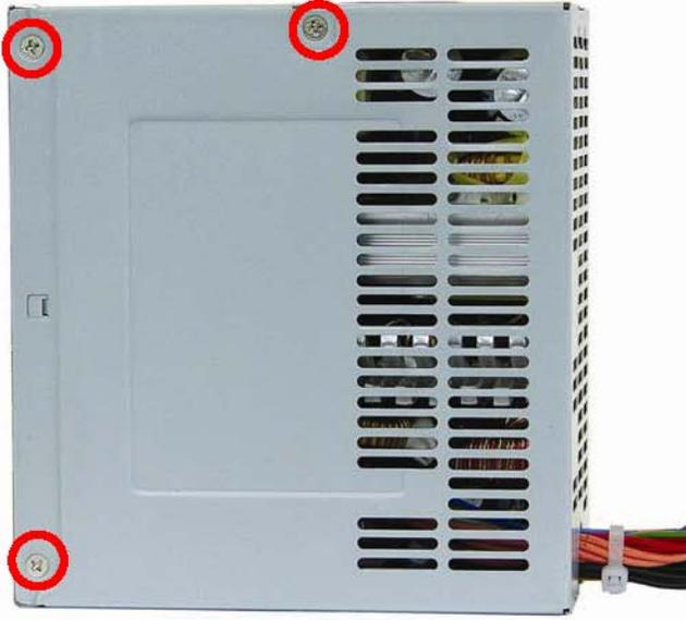
FIGURE 12: Power supply 2 – Plastic tie location
