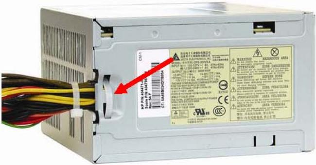
FIGURE 13: Power supply 2 – PCA screw locations
