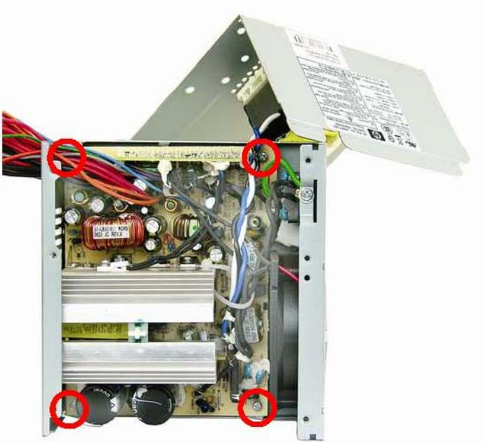
FIGURE 9: Power supply 1 –Capacitors and small PCA to cut
