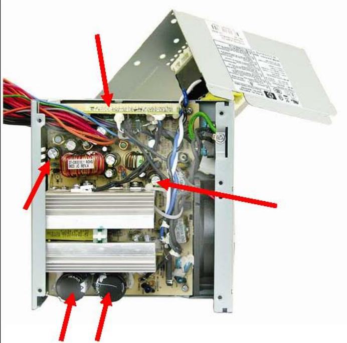
FIGURE 10: Power supply 2 –Cover screw locations
