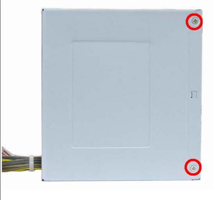
FIGURE 11: Power supply 2 – Cover screw locations
