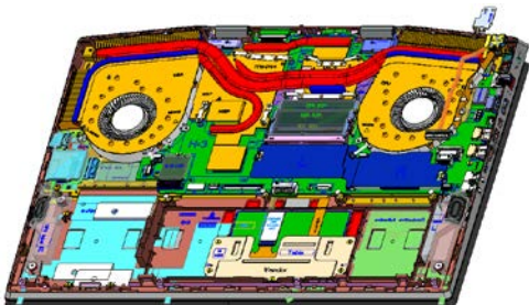
step 4, remove bracket and DC-in cable
