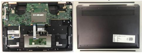
3.23 Remove black Mylar, battery, SSD, SSD shield can, Rear L/R fan, Power board
