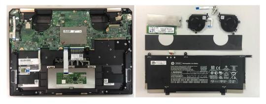
3.24 Remove Front L/R speaker, TP module ,Rear L/R speaker, FPR , FPR bracket ,FPR FFC , Audio board ,M/B
