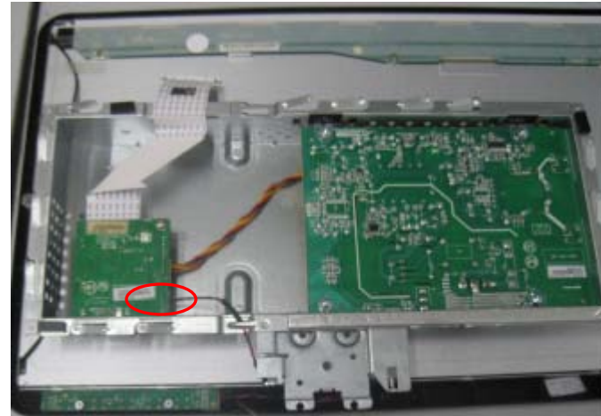
4.Remove key BD Connector from Interface BD
