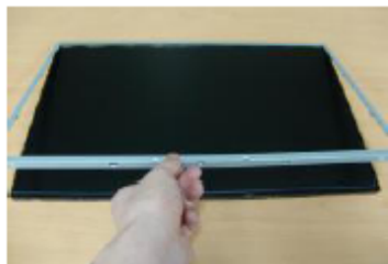
Step4 : Separate case top (push the case top because of damages on COF)
