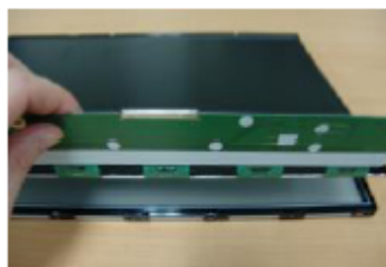
Step5 : Separate board ass'y
