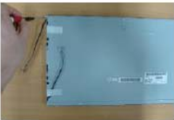
Step7 : Pull lamp housing with tool & hands (*Be careful not to break the Lamp)
