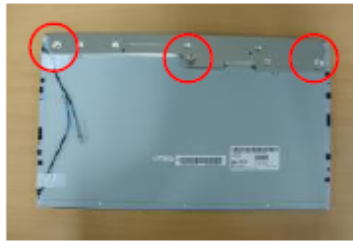
Step1: Unfix the Screw (3 Point) Remove the cover shield
